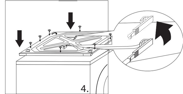
1) Position the unit on a level surface, capable of supporting the entire weight of the dryer. Remember that the unit will be heavier when it is fully loaded. Clean the surface where the stacking kit is going to be installed. Place the mounting bracket on the Washer as indicated.
